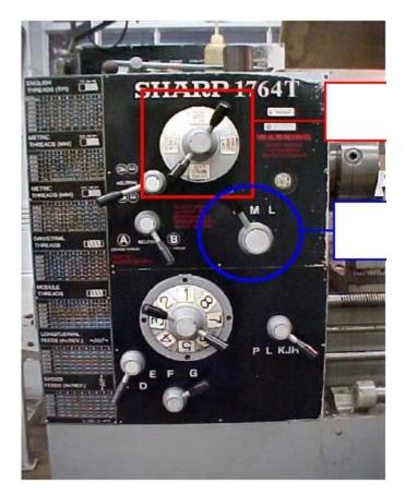
Shifting of spindle speed gears should be done with the spindle stopped and either manually turning the chuck by hand or using the control panel "JOG" button while moving the speed dial and/or speed range (high, medium and low) lever.
