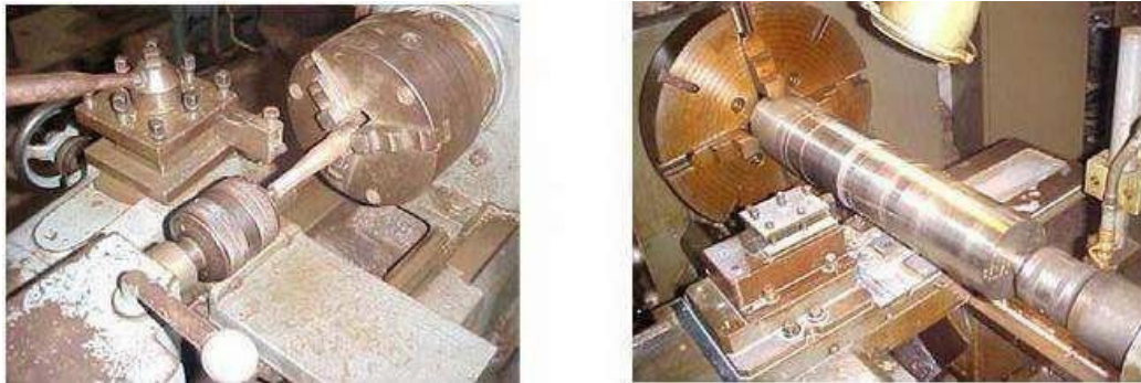
Fig. 2.19 Work held between chuck and revolving centre
