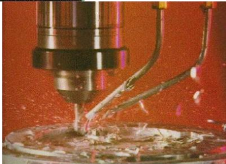
3.Mist :cutting fluid is atomised by a jet of air and the mist is directed at the cutting zone
