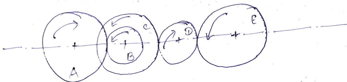
Speed ratio for gears A & B
