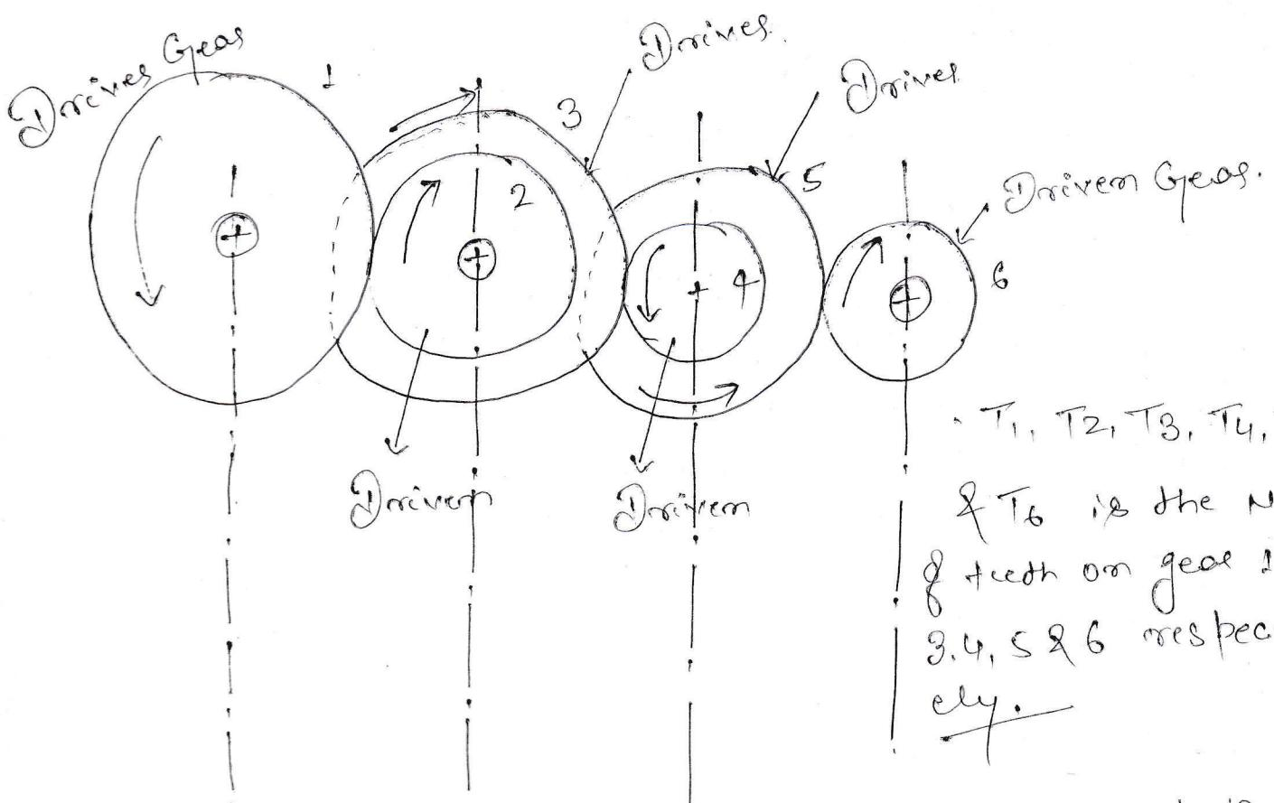
Gear 2 & Gear 3 is Compound gear because it is mounted on the same shaft.
