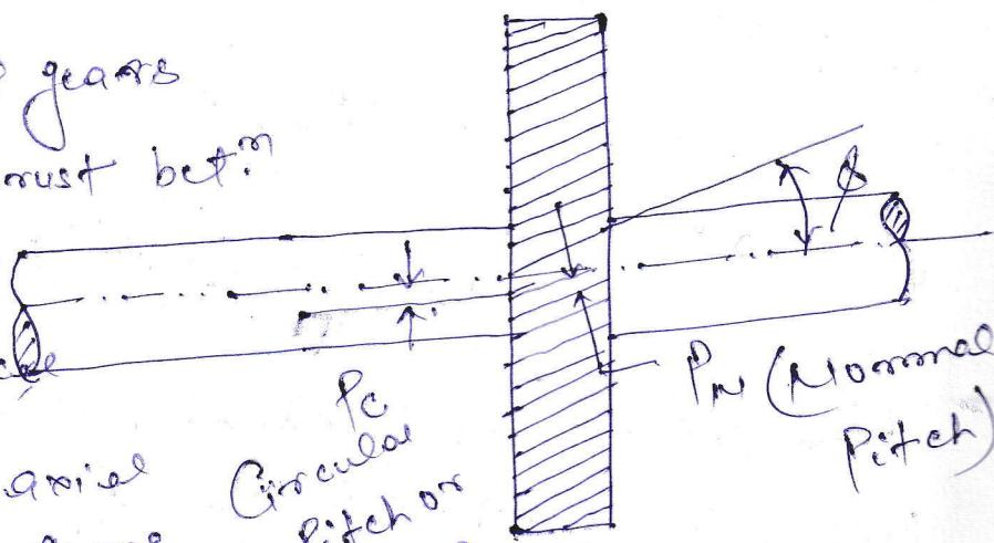
→ Centre distance for a pair of spiral gears:-
