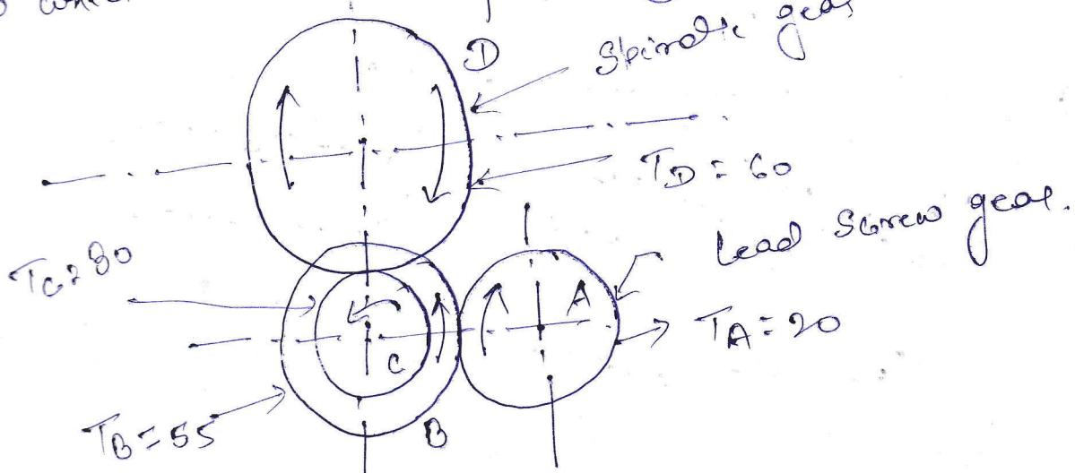
Q.No(4): Fig. shows a Compound gear train in which wheel A is fixed to the driving shaft, B-C are compounded, D is idle and E is fixed on the driven shaft. If gear A rotates at 1000 r.p.m. find the speed and direction of E.
