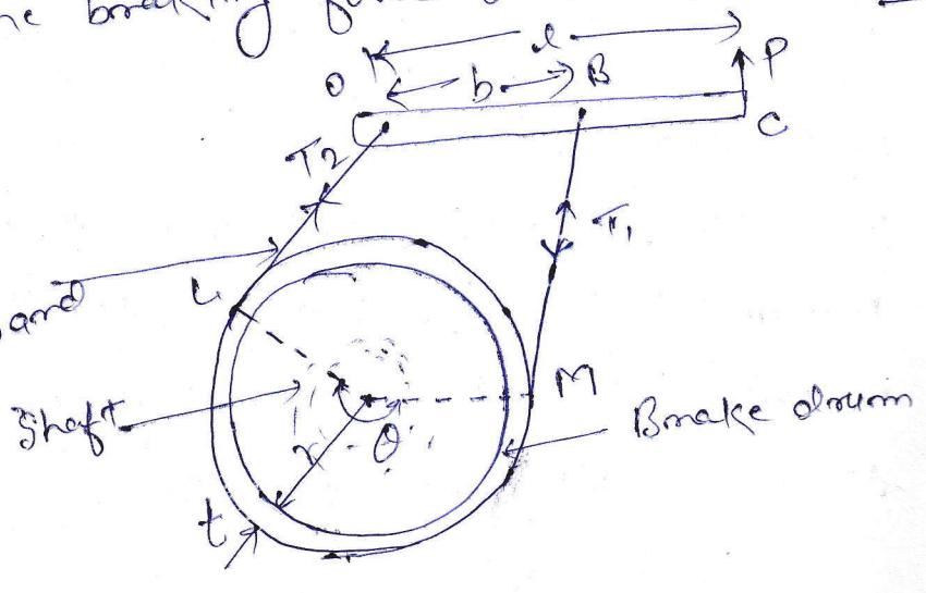
$\theta$ : Angle of wrap (embraze) of the band on the drum.
