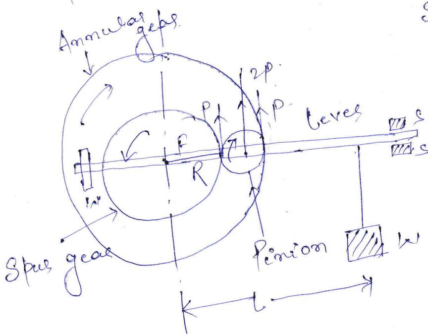
Spur gear attached to Engine Shaft (Driving Shaft) rotates in clockwise direction.
