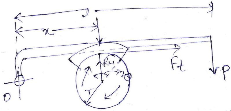
Braking torque for a Pivoted block or shoe brake is
