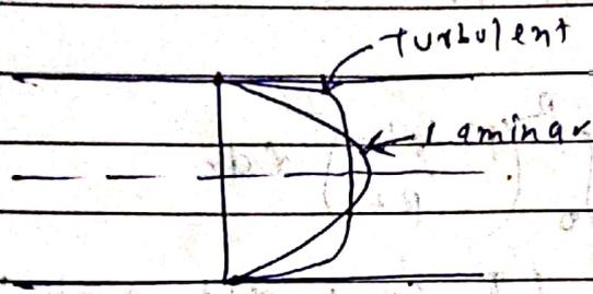
→ The lower correction factors for turbulent flow indicate that the velocity distribution is more uniform than in turbulent than in laminar flow.
