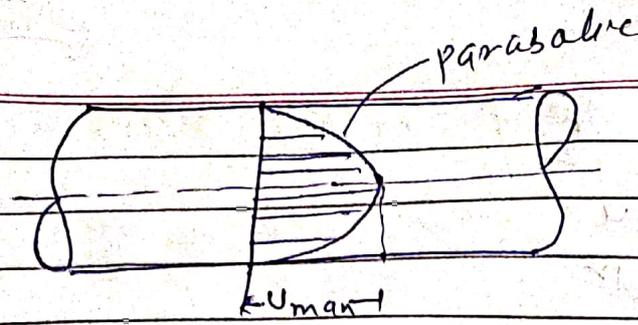
Discharge! → consider flow through an elemental ring of radius  $r$  and thickness  $dr$
