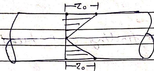
The shear stress increases linearly from zero at the center line of the pipe to the maximum at the pipe surface ( $r_0$ ).
