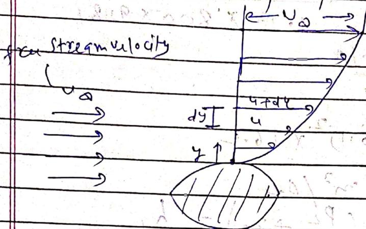
When a real fluid flows past a solid boundary a fluid on the surface will have same velocity as that of the surface if the boundary is static the fluid will also have zero velocity. Away from the boundary the fluid velocity gradually increases and velocity gradient  $\frac{du}{dy}$  exists in a region closed to the boundary. This region is known as Boundary layer region. Thus velocity gradient will give rise to shear stress and hence the flow is viscous in Boundary layer region.
