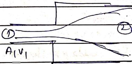
$$h_{L \text{ exp}} = \frac{(V_1 - V_2)^2}{2g}$$
