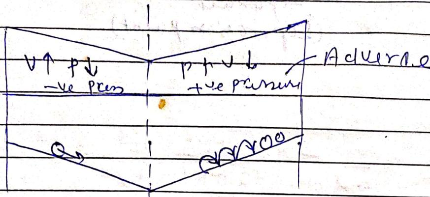
In case of convergent flow (accelerating flow) the velocity increases and pressure decreases therefore fluid slides down the pressure hill when the fluid flows through a divergent passage the velocity decreases and pressure increases therefore the fluid moves under the positive pressure gradient and hence the fluid has to climb a pressure hill. if the
