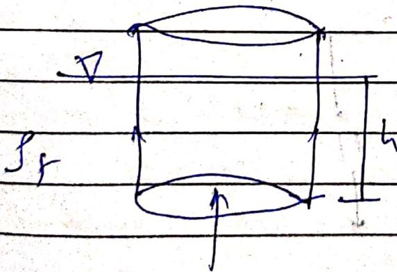
$$F_{net} = \rho_f g h A \leftarrow \begin{matrix} \text{vol of submerged or} \\ \text{vol of fluid displaced (V)} \end{matrix}$$
