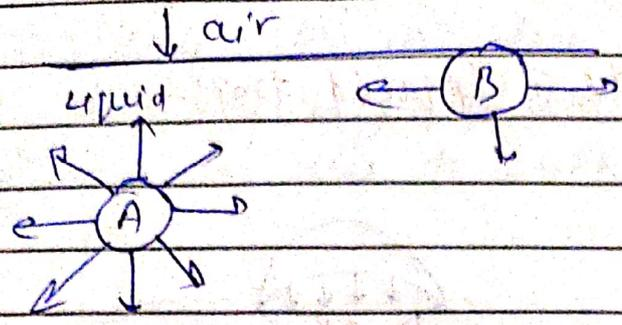
consider the molecule A which is below the free surface of the liquid this molecule surrounded by various corresponding molecule and because of various cohesive forces it will be under equilibrium.
