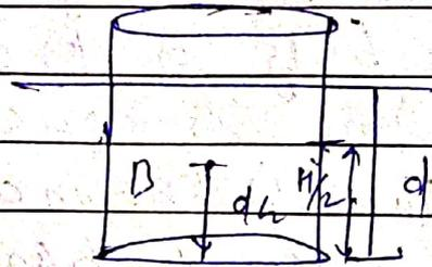
Principle of Floation!  $\rightarrow$  When a body is floating in a fluid wt of the body is equal to Buoyant force. But Buoyant force in turn is equal to wt of the fluid displaced, therefore for a floating body in equilibrium wt of Body is equal to wt of fluid displaced.
