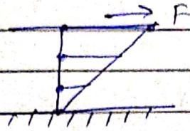
concretely a fluid is a substance which changes it's relative position under the action of shear force.
