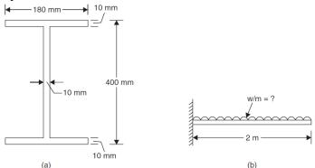
Q10. Compare the moment carrying capacity of the section given in Q.9 with equivalent section of the same area but (i) square section, (ii) rectangular section with depth twice the width and (iii) a circular section.
