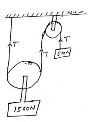
$F8.2 - f 1500 \times block$  EV = 0  $2T + f_{1} = 1500$   $2T + \frac{1500}{9.81} = 1500$   $2T + \frac{1500}{9.81} \times a = 1500$
