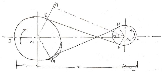
In a cross belt drive both the pulley notates in opposite directions
