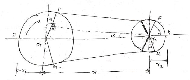
In the open belt drive both the pulleys rotates in the same direction.
