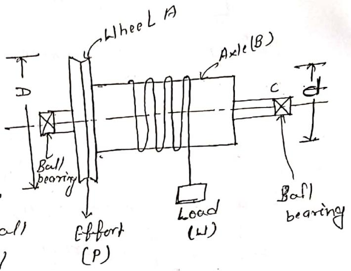
The load W to be lifted is attached to a string which is wound round the axle. Another string is wound round the wheel and the effort P is applied to it. These two strings are wound in opposite direction. which makes the load move upward when the effort is applied downward.
