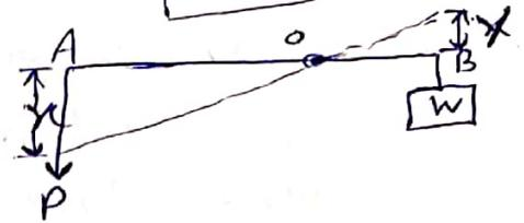
→ (M.A. > 1) → Mechanical advantage is always greater than one because the effort applied is generally smaller than the load lifted.
