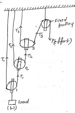
The load is affached to the bottom most pulley where as the effort is applied to the effort end of rope which passes round the upper most pulley.
