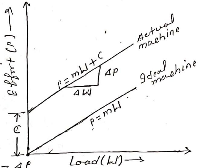
where,  $m = \text{slope of straight line} = \frac{\Delta P}{\Delta W}$
