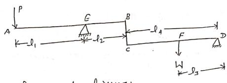
blith refrence to figure: AB is a simple lever connected to another simple lever CD with the help of a link BC. P is the effort
