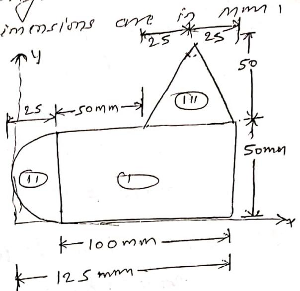
Sol<sup>n</sup>:- This section is not symmetrical about any axis therefore we have to find out the both the values  $\bar{x}$  and  $\bar{y}$ .
