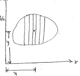
of on area of possing figure with respect to an axis perpendicular to the (u-y) plane and possing through a pole (z-axis) is called polar moment of inertia and is denoted by Izz or Jo.
