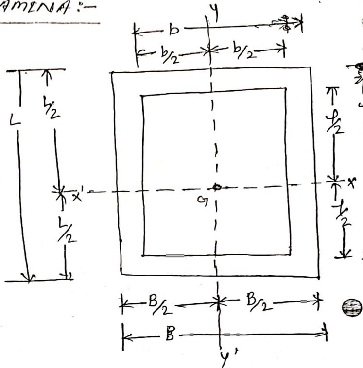
Rectangular lamina of length ( $L$ ) and width ( $B$ ) has rectangular slot of length ( $l$ ) and width ( $b$ ). Area moment of inertia about centroidal axis can be given as -
