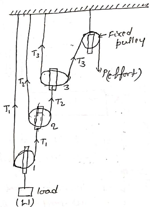
→ The load is attached to the bottom most pulley where as the effort is applied to the effort end of rope which passes round the upper most pulley.
