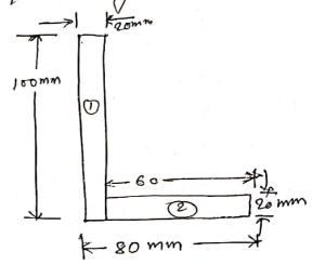
Pretample (1)  $q_1 = 100 \times 20 = 2000 \text{ mm}^2$   $2l_1 = \frac{20}{2} = 10 \text{ mm}$   $y_1 = \frac{100}{2} = 50 \text{ mm}$
