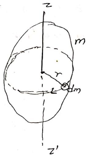
consider a rigid body of mass M. Take an element of a mass (dm) at a distance (r) from the axis as shown in fig. Here (r) is the moment of arm.
