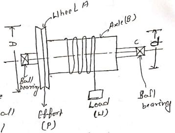
and gale can be rotated. The load W to be lifted is attached to a string which is wound round the axle. Another string is wound round the wheel and the effort p is applied to it. These two strings are wound in opposite direction. which is makes the load move upward when the effort is applied downward.
