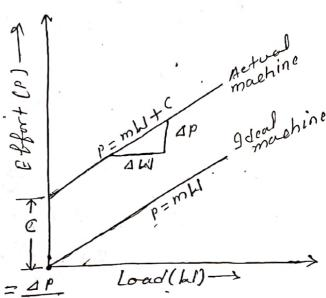
where, m = slope of straight line = 1P e = Intercept of the line on p-axis.
