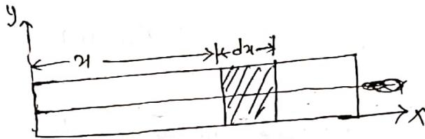
When the  $x$ -axis is so chosen that it passes through the centre of the wire and along its length  $\bar{y} = 0$
