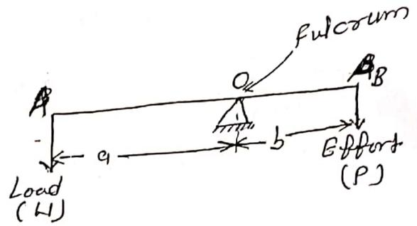
The perpendicular distance of point A, at which load is applied from the fulcrum (O) is called load arm ( $OA = a$ ).
