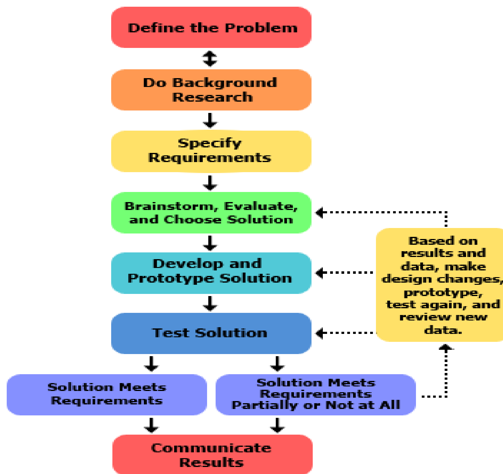
Fig. Steps of Mechanical Engineering Machine Design
