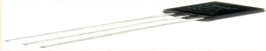
fig: Temperature Sensor Major Applications: mainly includes refrigerators, AC's etc.
