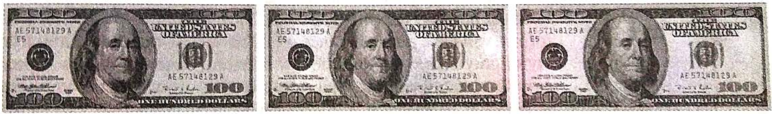
FIGURE 3.15 Images reconstructed using (a) bit planes 8 and 7; (b) bit planes 8, 7, and 6; and (c) bit planes 8, 7, 6, and 5. Compare (c) with Fig. 3.14(a).
