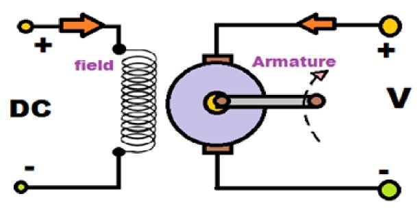
In this, the armature and field windings of a separately excited DC motor is fed with separate D.C. power source.
