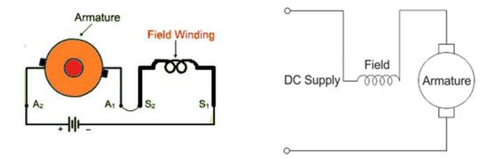
The field winding is connected in series to the armature winding. Thus the field winding are exposed to the entire armature current unlike in the case of a shunt motor. The motor speed varies as a non-linear function of load torque and armature current. This motor is used when high starting torque is desirable.
