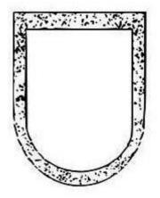
• Semi-circular shaped sewer: In this type of sewer, the outer surface is circular. The inner surface is divided into two portions. The upper portion resembles a basket-handle and the lower portion is like a channel. During dry season, the sewage flows through the lower portion and during monsoon, the combined sewage flows through the full section.
