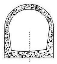
Parabolic shaped sewer
