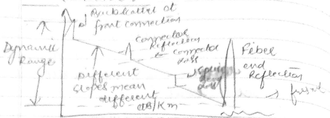
Representation trace of backscattered reflected optical power as displayed on an OTDR screen and the meaning of various trace features.
