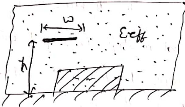
Fig.:- Equivalent geometry of micro strip line.
