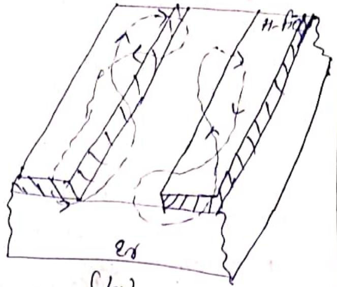
fig. (a) E-field in slot line, (b) H-field in slot line.
