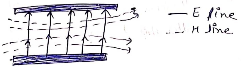
Fig. 2:- TEM field pattern in parallel stripline
