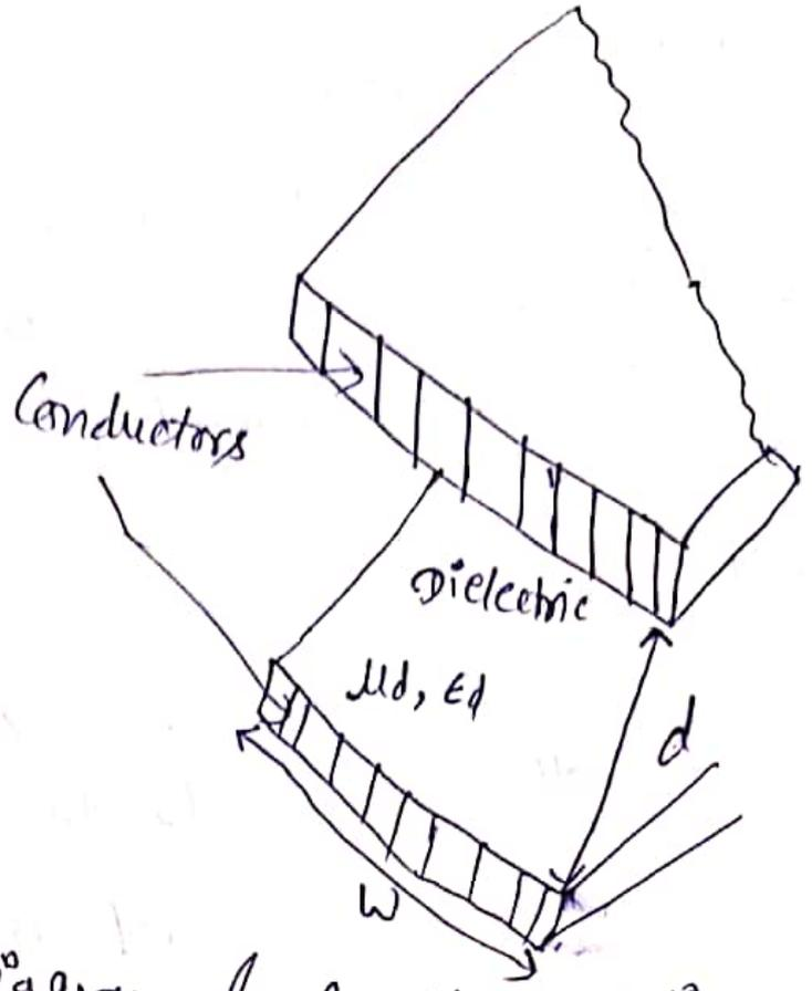
Fig. 1:- Schematic diagram of parallel stripline
