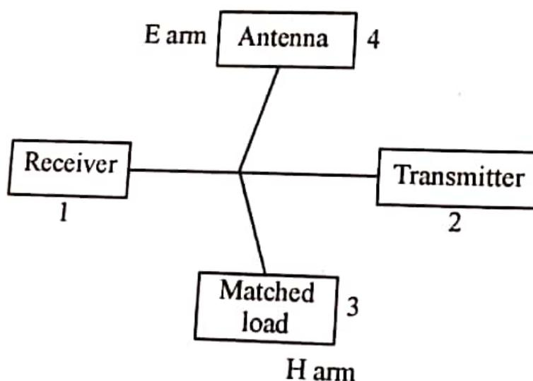
Figure 5.9 Magic Tee in Antenna duplexer
