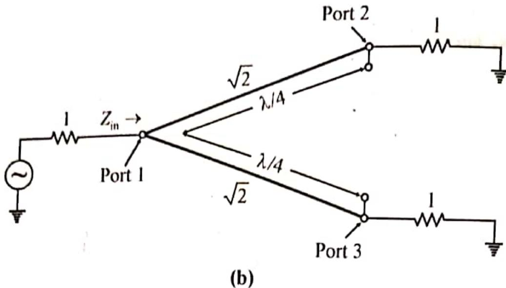
Figure 6.36 Analysis of the Wilkinson divider to find  $S_{11}$  (a) The terminated Wilkinson divider (b) Bisection of the circuit in (a)
