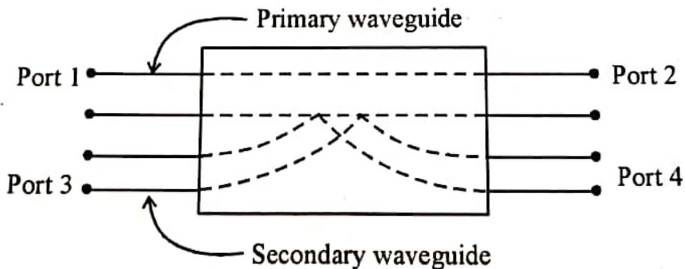
**Figure 5.13 Schematic of directional coupler**
