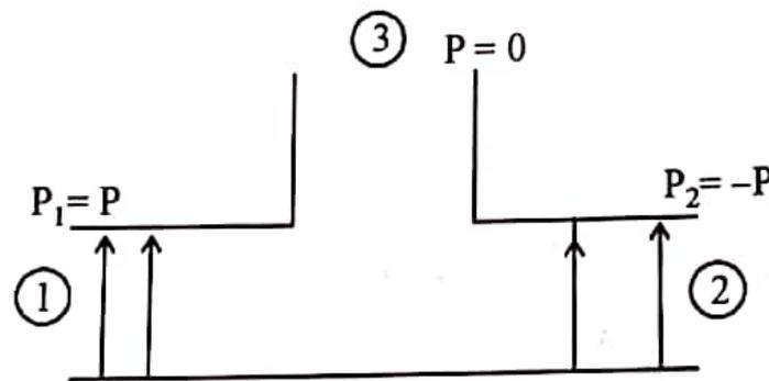
Figure 5.6 (b) Zero output at port (3) if power fed from port (1) & (2) are in same phase and same in amplitude
