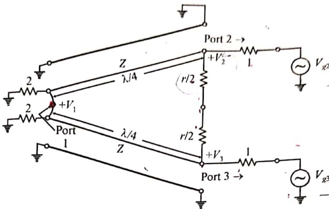
Figure 6.34 The Wilkinson power divider circuit in normalized and symmetric form
