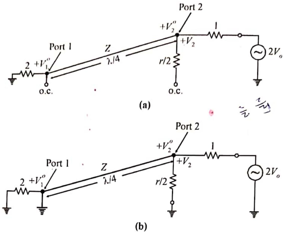
Figure 6.35 Bisection of the circuit of figure 6.34 (a) Even-mode excitation (b) Odd-mode excitation
