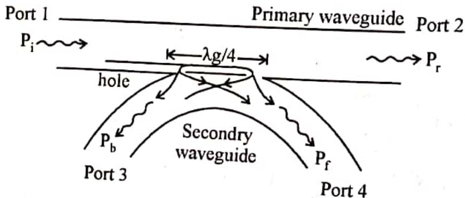
Figure 5.16 Two hole directional coupler
