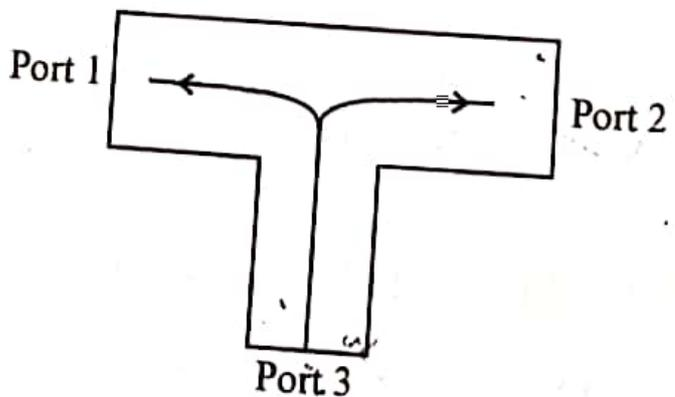
Figure 5.3 Top view of H plane waveguide tee
