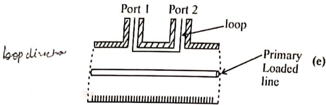
Figure 5.15 (a) Two hole cross guide directional coupler (b) Two hole branches guide couplers. (c) short slot coupler (d) Bifurcated coupler (e) Loop directional coupler.
