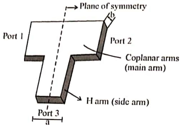
Figure 5.2 Structure of H plane Tee
