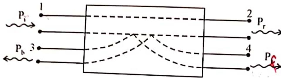
Figure 5.14 Directional coupler indicating power
