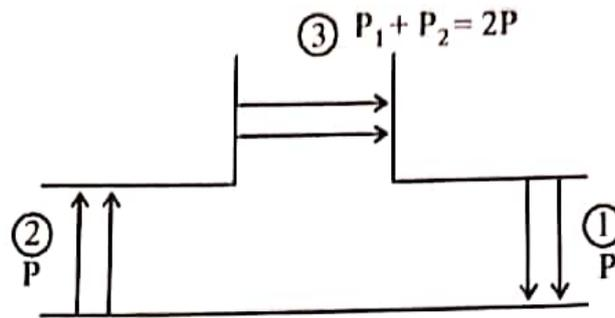
Figure 5.6 (a) Output is doubled at port (3) if power fed from port (1) & (2) are opposite in phase and same in amplitude.
