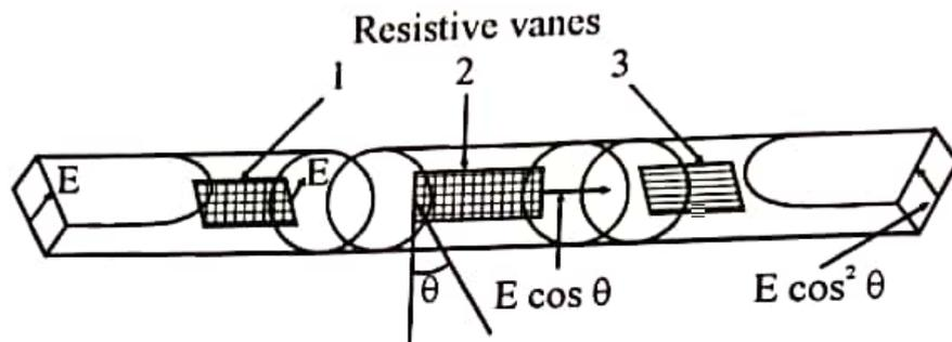
**Figure 5.21 Rotary wave precision attenuator**
