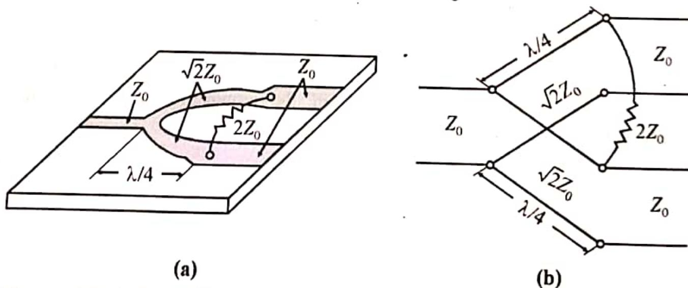
Figure 6.33 The Wilkinson power divider (a) An equal-split Wilkinson power divider in microstrip line from (b) Equivalent transmission line circuit
