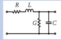
➢ But for no reflection, Y<sub>s</sub>=G<sub>s</sub>+jB<sub>s</sub>=1+j0  $\frac{Y_r(1+\tan^2\beta L_s)}{1+Y_r^2\tan^2\beta L_s} = 1$ L<sub>s</sub>-distance of stub from load
