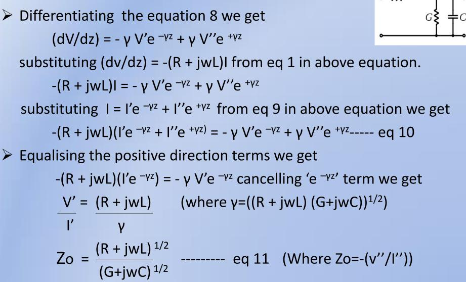
Value of Zo doesn't depend upon the length of transmission line but on R,L,G and C.
