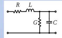
as  $\gamma = \alpha + j\beta$  where  $\alpha$  – attenuation factor,  $\beta$ -phase velocity
