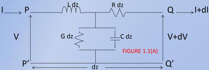
When current is flowing in 2 parallel wire magnetic field will get induced around the wire so there will be inductance known as loop inductance(H/km) whose value depend upon the strength of current so it is in series with loop resistance.
