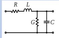
Input impedance at any point of transmission line is given by  $Zin = \frac{Zo(Z_{R} + Zo tanh(\gamma L))}{Zo + Z_{R} tanh(\gamma L)}$ Now converting impedance to admittance by  $Y_0 = 1/Z_0$  [Characteristic admittance]  $Y_{R}=1/Z_{R}$  [Load admittance] Y<sub>in</sub>=1/Z<sub>in</sub> [input admittance]  $Y_s = Y_o \frac{Y_R + Y_o tanh(\gamma L)}{Y_o + Y_P tanh(\gamma L)}$
