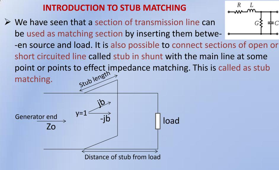
Real part will be matched by position(should move stub from load).
