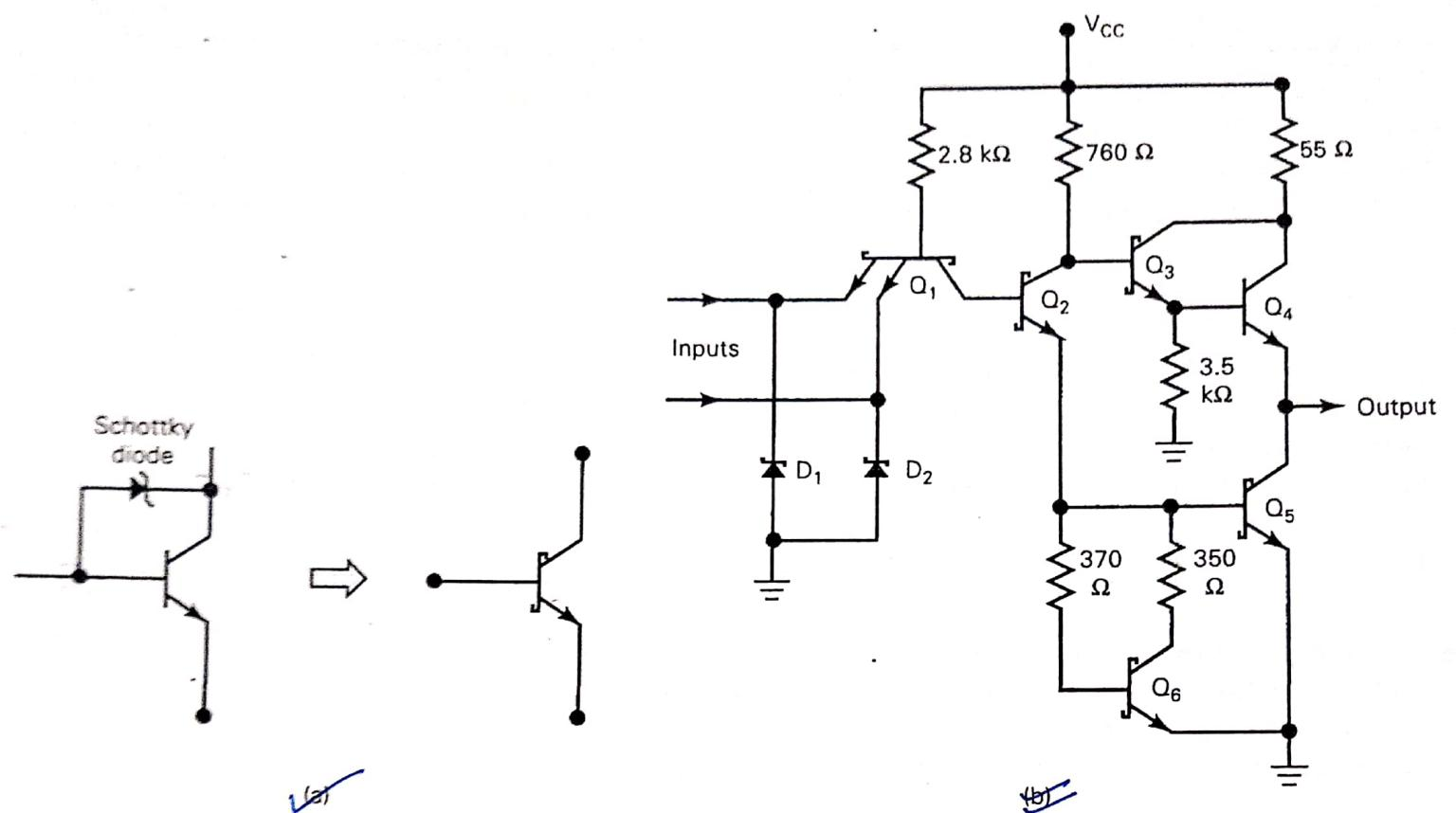
FIGURE 8-12 (a) Schottky-clamped transistor; (b) basic NAND gate in S-TTL series. (Courtesy of Fairchild, a Schlumberger company)
