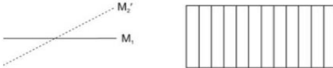
Fig. 4: Formation of straight line fringes
