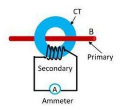
The line current is too high, and it is very difficult to measure them directly. Thus, the current transformer is used which decrease the high value of current into a fractional value which is easy to measure by the instrument.
