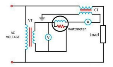
The primary terminal of the potential transformer is connected to the line for measuring the line voltage. The potential transformer reduced the high value of voltage into the small value which can easily be measured by the voltmeter or meter.
