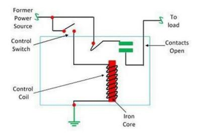
This magnetic field moves the relay armature for opening or closing the connections. The small power relay has only one contacts, and the high power relay has two contacts for opening the switch.
