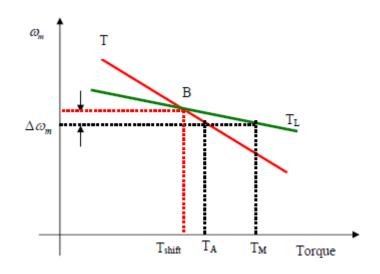
Inequality in the above equation can be derived by an alternative approach. Let a small perturbation in speed,  $\Delta m$  results in  $\Delta T$  and  $\Delta T_1$  perturbation in T and T1 respectively. Therefore the general load torque equation becomes
