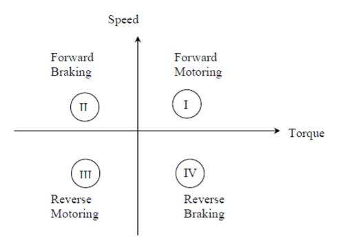
In quadrant I, developed power is positive, hence machine works as a motor supplying mechanical energy. Operation in quadrant I is therefore called Forward Motoring.
