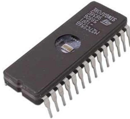
Figure : A typical EPROM chip
