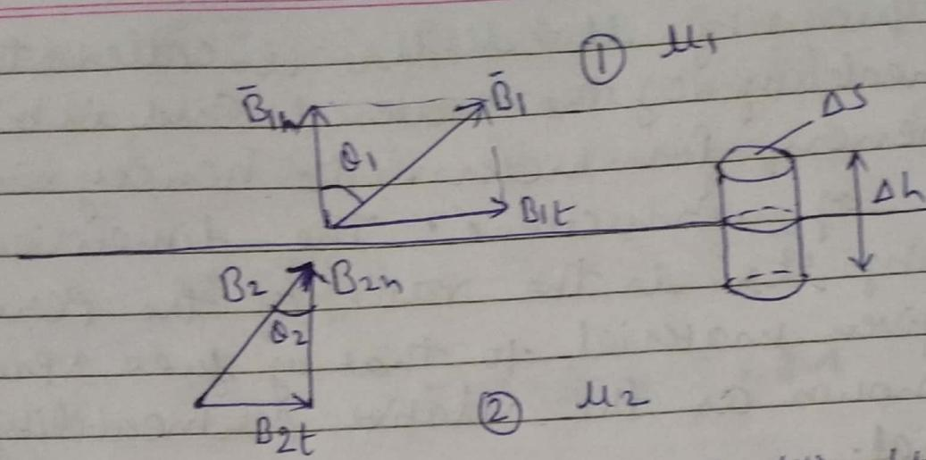
fig (a) Boundary condition b/w two magnetic media for  $\vec{B}$
