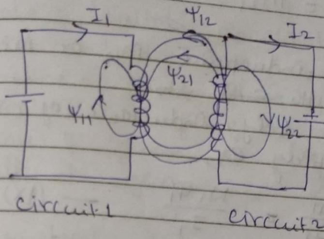
fig (b) magnetic induction b/w two circuit-s.
