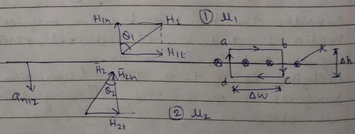
fig (b) Boundary conditions b/w two magnetic media for  $\vec{H}$
