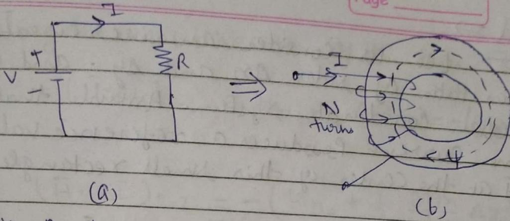
fig- Analogy b/w (a) an electric circuit and (b) a magnetic circuit.
