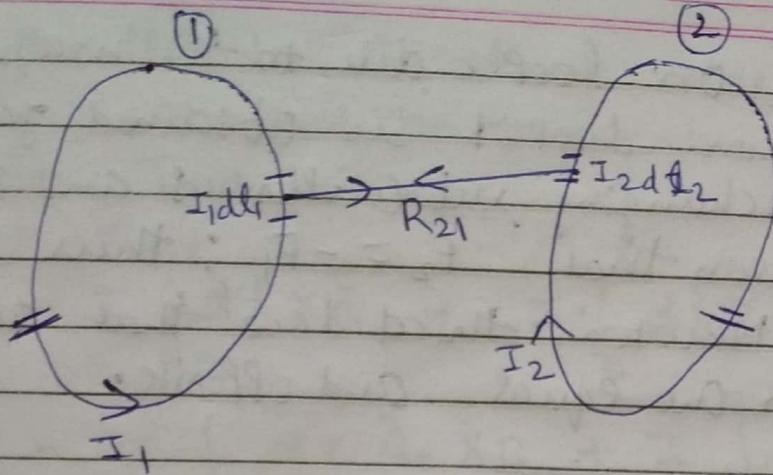
Fig - Force b/w two current loops
