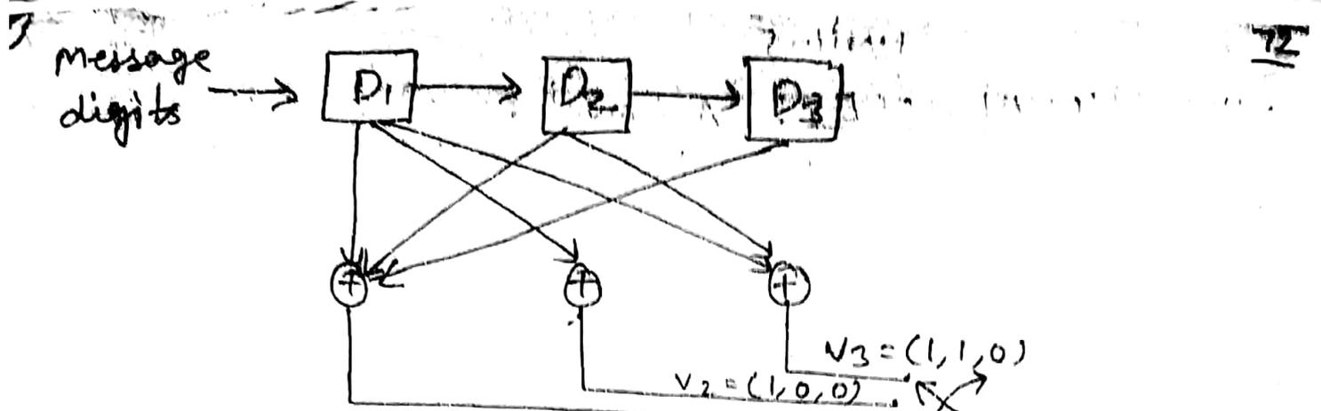
This (3,1,3) Convolutional Encoder has 3 memory registers, 1 input bit and 3 output bits.
