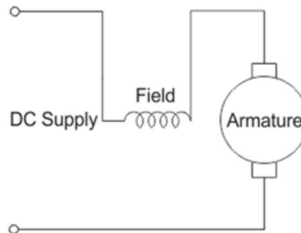
The field winding is connected in series to the armature winding. Thus the field winding are exposed to the entire armature current unlike in the case of a shunt motor. The motor speed varies as a non-linear function of load torque and armature current. This motor is used when high starting torque is desirable.
