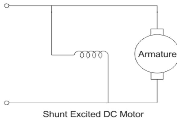
The supply current in case of the **shunt wound DC motor** is split up into 2 parts.  $I_a$ , flowing through the armature winding of resistance  $R_a$  and  $I_{sh}$  flowing through the field winding of resistance  $R_{sh}$ . The voltage across both windings remains the same.
