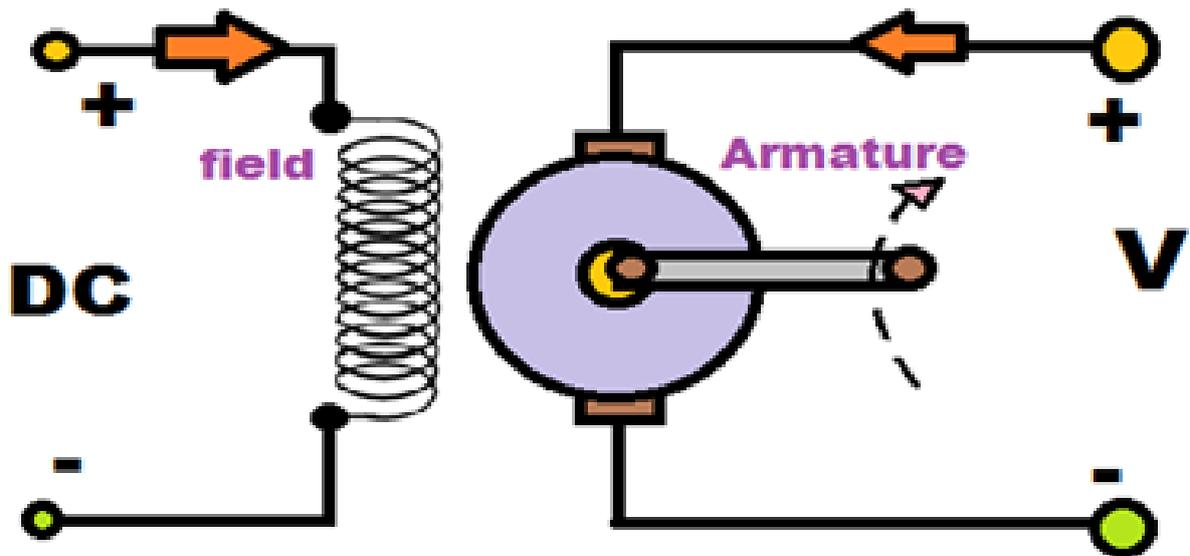
In this, the armature and field windings of a separately excited DC motor is fed with separate D.C. power source.
