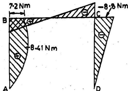
Figure 11.33 : Bending Moment Diagram
