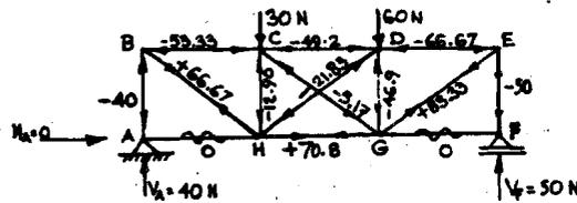
Figure 11.5 (f) : Final Member Forces in the Truss
