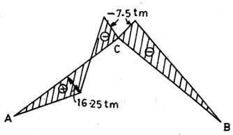
Figure 11.36 : Bending Moment Diagram
