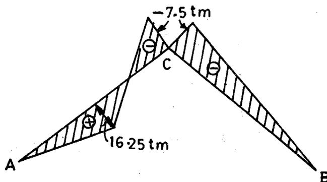
Figure 11.36 : Bending Moment Diagram
