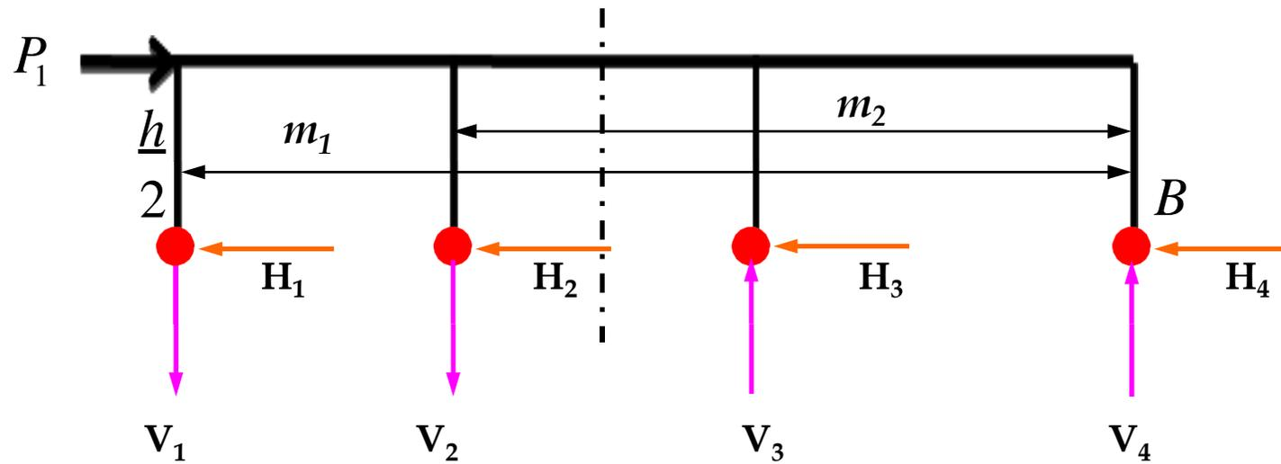
$$\sum M_B \Rightarrow P_1 \frac{h}{2} = V_1 m_1 + V_2 m_2 - V_3 m_3 - V_4 m_4 \quad \text{_____} (2)$$
