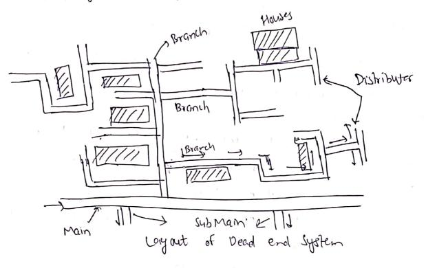
Advantage: - checip in initial last and easty determination of pipe diameters, values etc.
