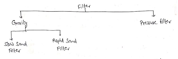
=) Gravity filters are those filter in which head required by water to flow through the filter medium is provided by Height of water itself above the filter medium, where as in core of pressure filter the head is provided artificial by the external application of pressure over the filter medium.
