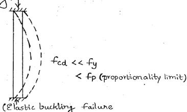
(Elastic buckling failure in long column)
