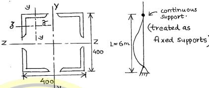
Design axial compressive load,  $P = fcd \times Ae$ .
