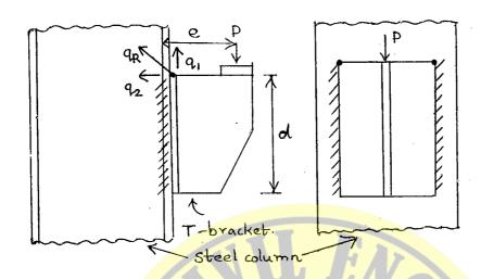
Ventical shear stress in weld due to P is q1,
