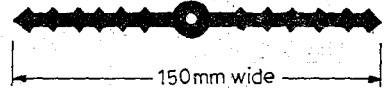
(d) 150 mm wide PVC water stop serrated with central bulb for construction joints.
