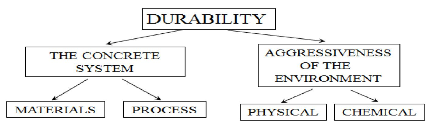
Binder type Binder content Aggregates Admixture Mixture design Mixing Transporting Compaction Curing Temperature Workmanship
