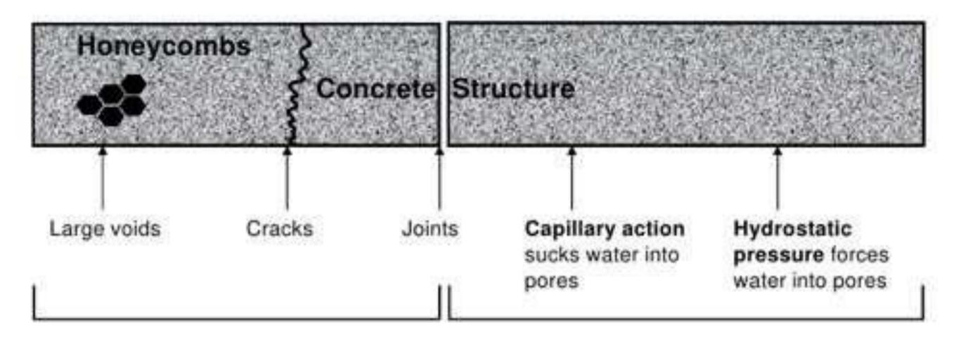
Penetration through Openings Penetration through Concrete
