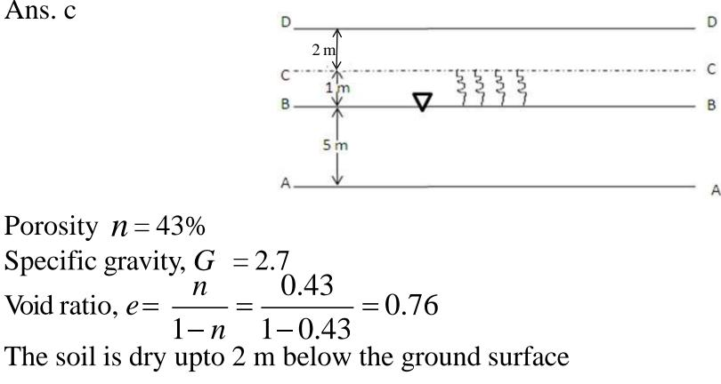
$$\gamma_d = \frac{G\gamma_w}{1+e} = \frac{2.7 \times 10}{1+0.76} = 15.34 \,\mathrm{kN/m^3}$$
