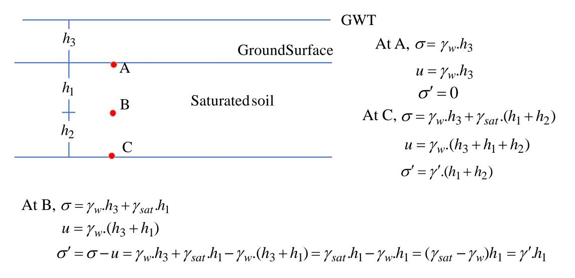
total pressure and pore water pressure increases by the same amount and hence no change in effective stress at any point below the ground.
