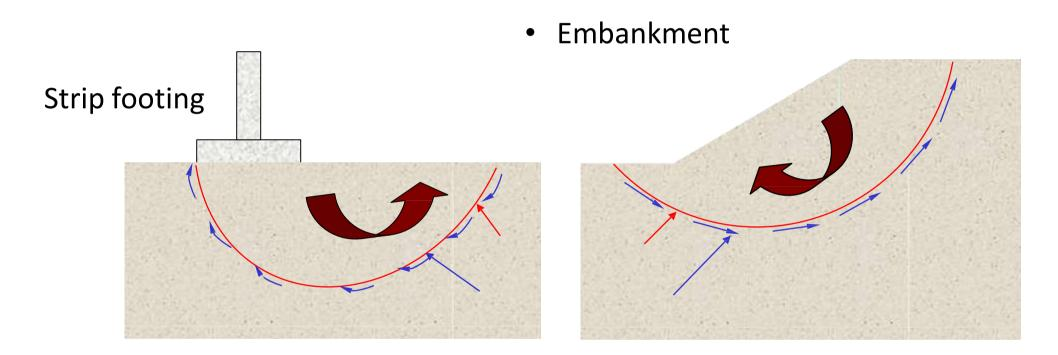
Failure surface Mobilized shear resistance
