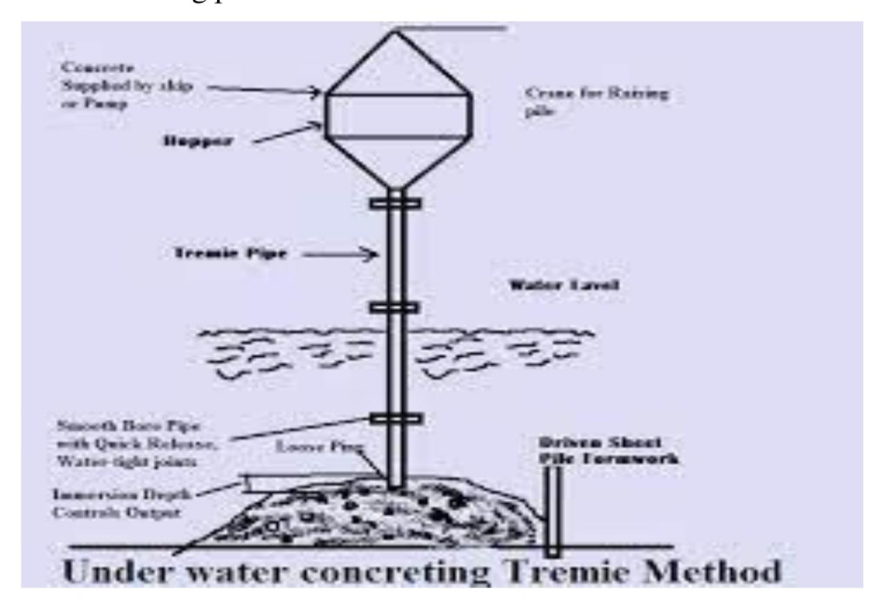
Underwater Concreting The underwater concreting techniques designed mostly to prevent cement washout. Methods to carry out underwater concreting:
