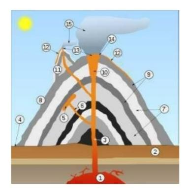
1. Large magma chamber 2. Bedrock 3. Conduit (pipe) 4. Base 5. Sill 6. Dike 7. Layers of ash emitted by the volcano 8. Flank 9. Layers of lava emitted by the volcano 10. Throat 11. Parasitic cone 12. Lava flow 13. Vent 14. Crater 15. Ash cloud
