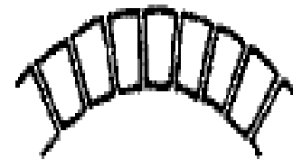
bricks cut to a wedge shape and mortar joints of uniform thickness
