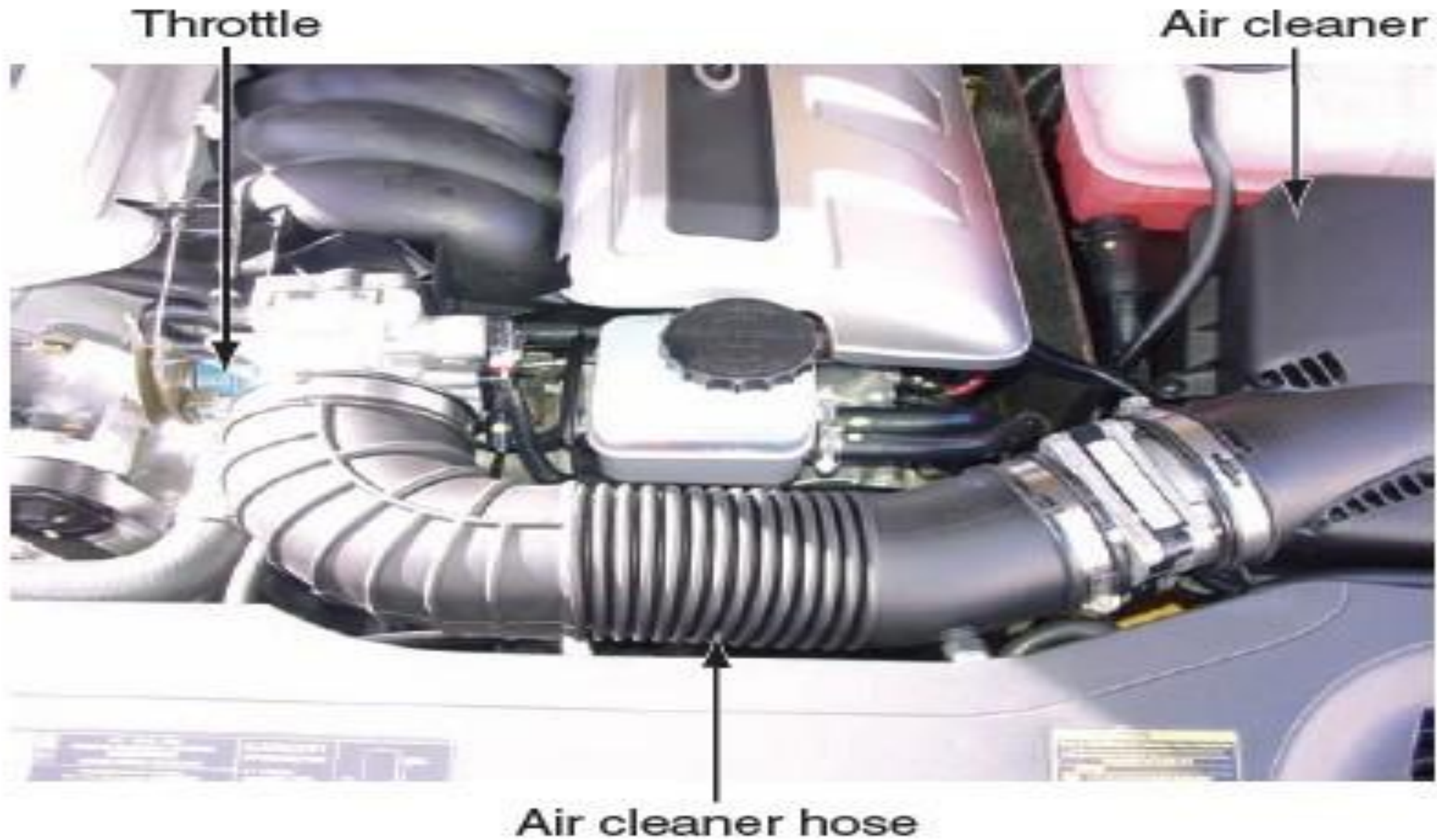
Figure 50.1 Remove the air cleaner and hose. Be careful not to crack the hose.
