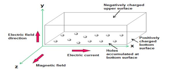
The Hall effect describes the behavior of the free carriers in a semiconductor when applying an electric as well as a magnetic field. The experimental setup shown in Figure, depicts a semiconductor bar with a rectangular cross section and length L. A voltage Vx is applied between the two contacts, resulting in a field along the x-direction. The magnetic field is applied in the z-direction.
