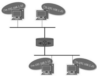
IP addressing provides mechanism to differentiate between hosts and network. Because IP addresses are assigned in hierarchical manner, a host always resides under a specific network. The host which needs to communicate outside its subnet, needs to know destination network address, where the packet/data is to be sent.
