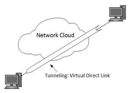
When the data enters from one end of Tunnel, it is tagged. This tagged data is then routed inside the intermediate or transit network to reach the other end of Tunnel. When data exists the Tunnel its tag is removed and delivered to the other part of thenetwork.
