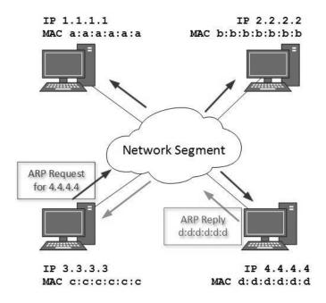
To know the MAC address of remote host on a broadcast domain, a computer wishing to initiate communication sends out an ARP broadcast message asking, "Who has this IP address?" Because it is a broadcast, all hosts on the network segment (broadcast domain) receive this packet and process it. ARP packet contains the IP address of destination host, the sending host wishes to talk to. When a host receives an ARP packet destined to it, it replies back with its own MAC address.
